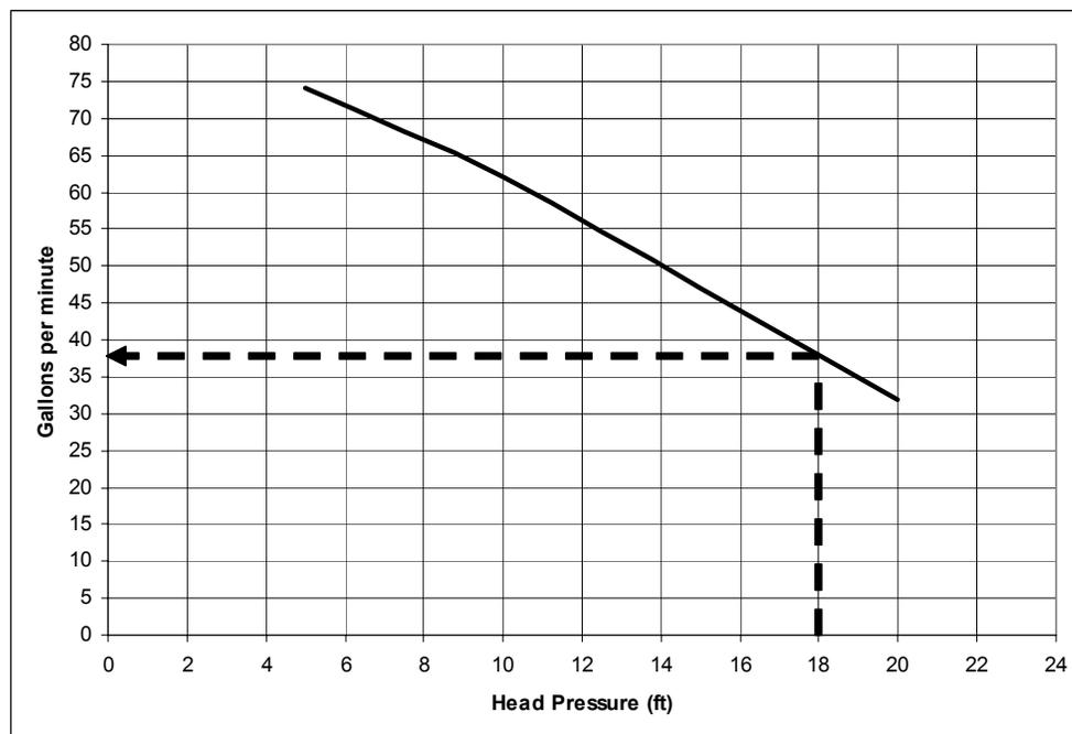
Figure 2. Water flow vs. Head Pressure for popular ½ hp submersible pump.
