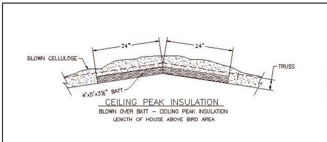
Figure 8. Ceiling peak insulation.
