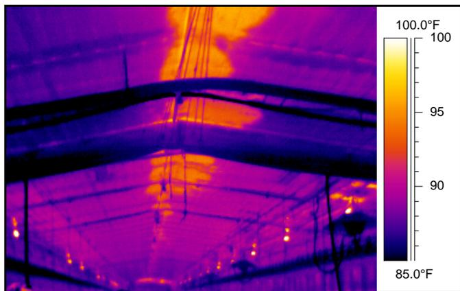
Figure 5. Thermal image of missing ceiling insulation taken during hot weather.
