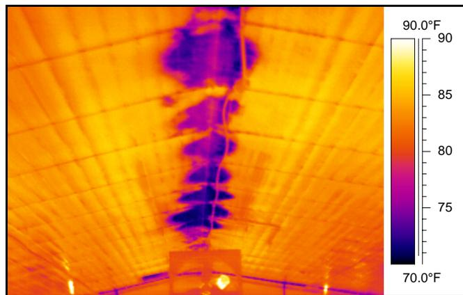
Figure 4. Thermal image of missing ceiling insulation.
