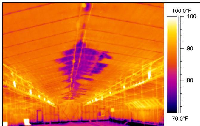
Figure 3. Thermal image of missing ceiling insulation taken during cold weather.
