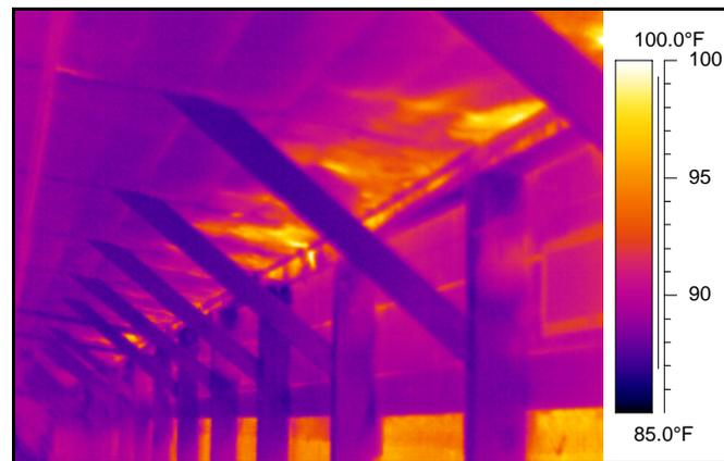
Figure 6. Missing ceiling insulation near side wall.
