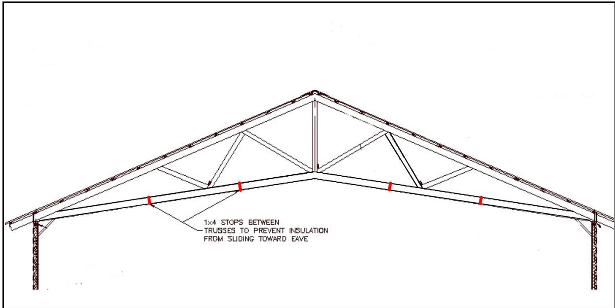
Figure 9. Ceiling insulation stops
