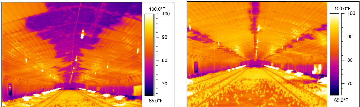
Figure 3. Thermal images taken during brooding in houses that were not reinsulated with the stabilized fiberglass insulation.
