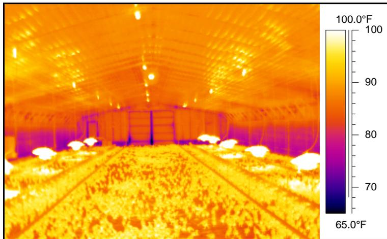
Figure 4. Thermal image of one of the houses after being reinsulated with the blown stabilized fiberglass insulation.
