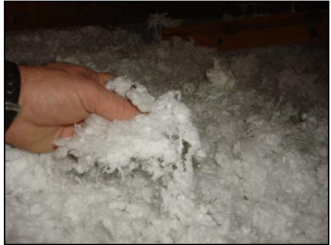
Figure 1. Blown stabilized fiberglass insulation.
