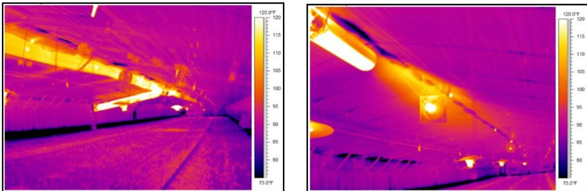
Figure 8. Thermal images of perforated duct and circulation fan heat delivery system in operation.
