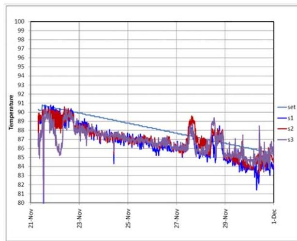
Figure 12. Temperature in control house with conventional radiant brooder heating system during brooding
