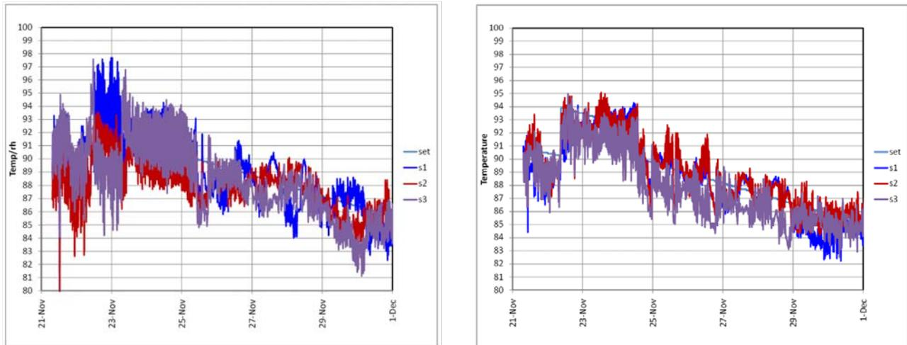
Figure 11. Temperatures in houses with alternative heating systems during brooding (Perforated duct delivery system - left, Circulation fan delivery system - right)
