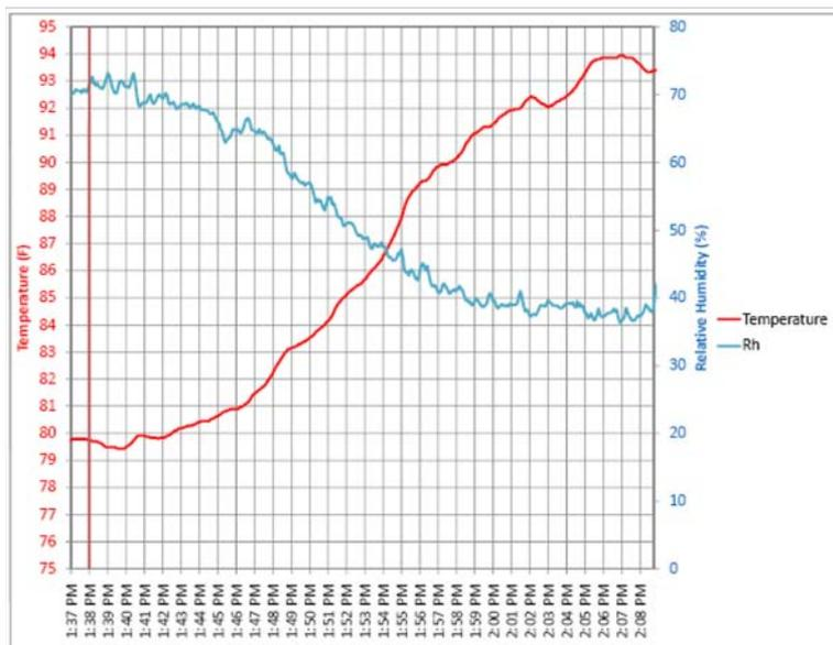
Figure 3. Cooling and Rh produced by a pad as it is drying.
