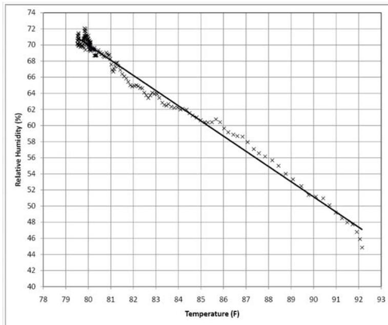
Figure 2. Temperature vs. Relative humidity of the air entering through a wetted pad.
