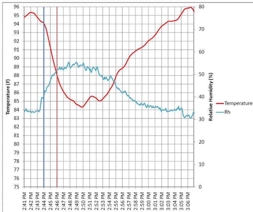
Figure 5. Pad system circulation pumps operating for two minutes.
