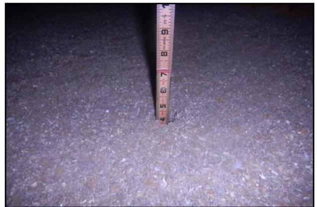
Figure 3. Blown cellulose insulation (February, 2011. Two years, six months after installation)
