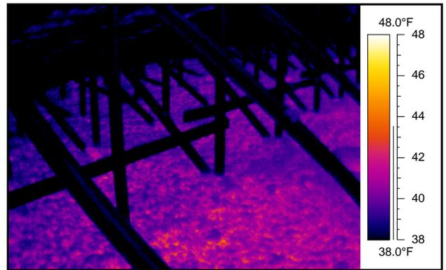
Figure 7. Thermal image of blown fiberglass insulation.
