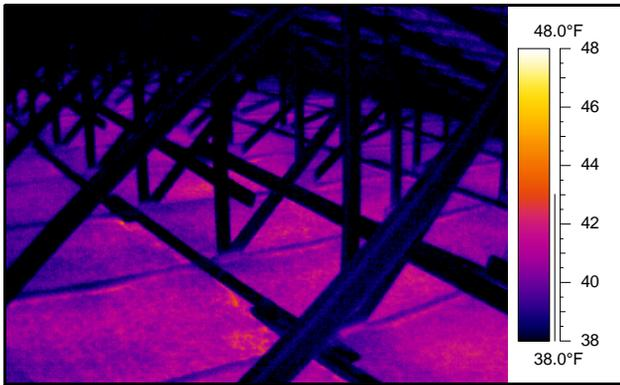
Figure 6. Thermal image of blown cellulose insulation.
