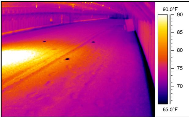
Figure 11. Floor heating pattern of GSI AV heater®.
