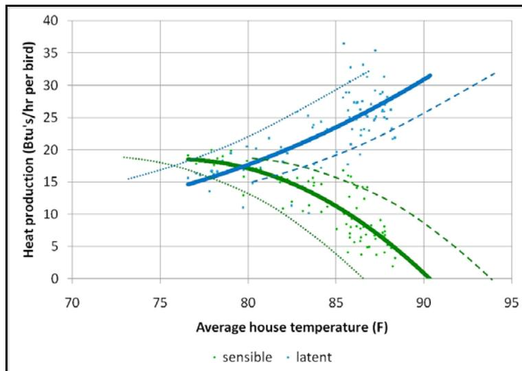
Figure 6. Sensible and latent heat loss as a function of house temperature.
