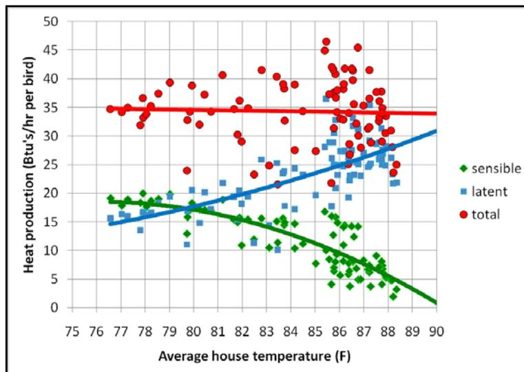
Figure 5. Sensible, latent, and total heat loss as a function of house air temperature.
