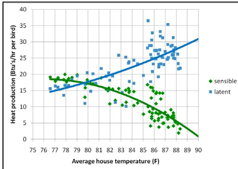
Figure 4. Sensible and latent bird heat removal
