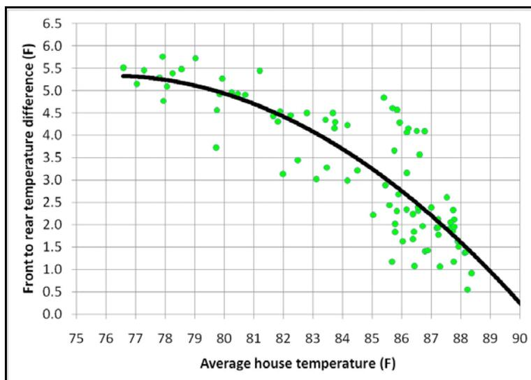
Figure 3. Temperature difference between inlet and exhaust ends
