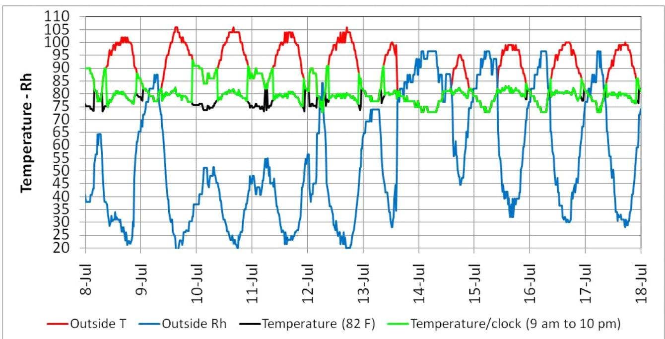
Figure 3. Comparison of house air temperatures with different evaporative cooling pad control schemes.
