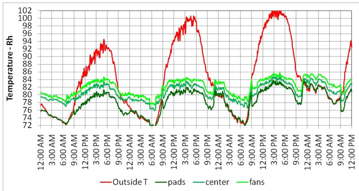
Figure 5. House temperatures in house where evaporative cooling pads are shut off between 10 pm and 10 am (August, 1 - 3).
