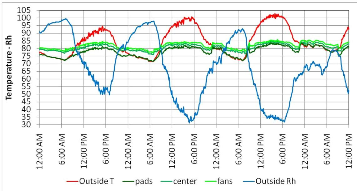
Figure 4. House temperatures in house where the pads are shut off between the hours of 10 pm and 10 am (Athens, Georgia August 1 - 3).
