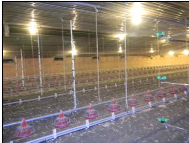
Figure 2. Anemometer poles in 60' wide house.
