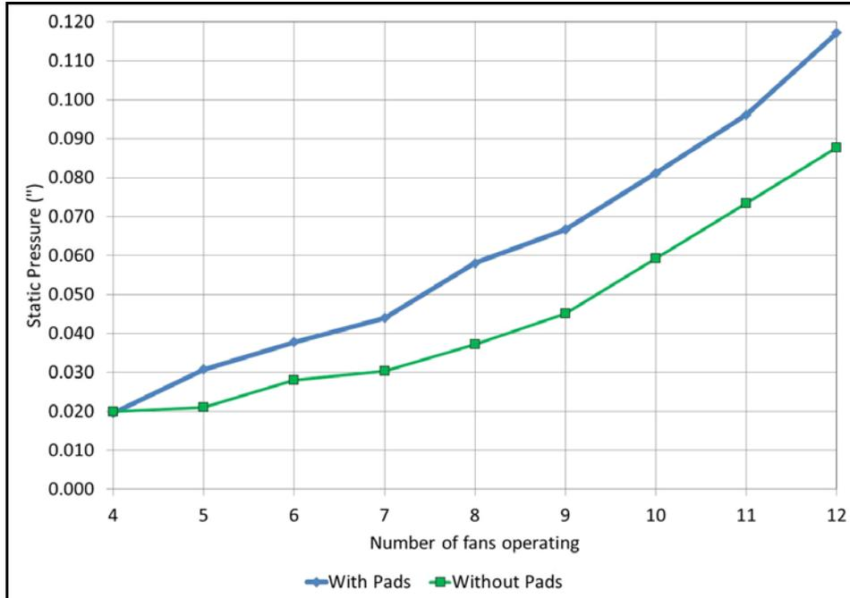
Figure 3. Fan static pressure with and without evaporative cooling pads.
