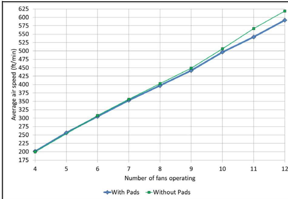
Figure 2. Average air velocity with and without evaporative cooling pads.
