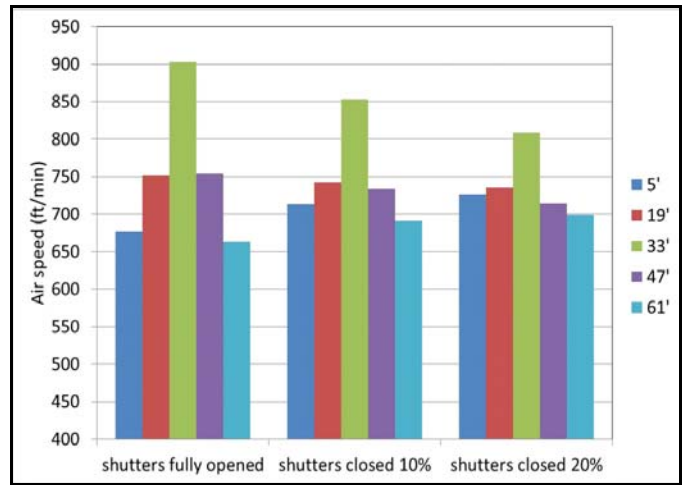
Figure 11. Air speed across width of house with all fans operating and tunnel shutters partially closed.
