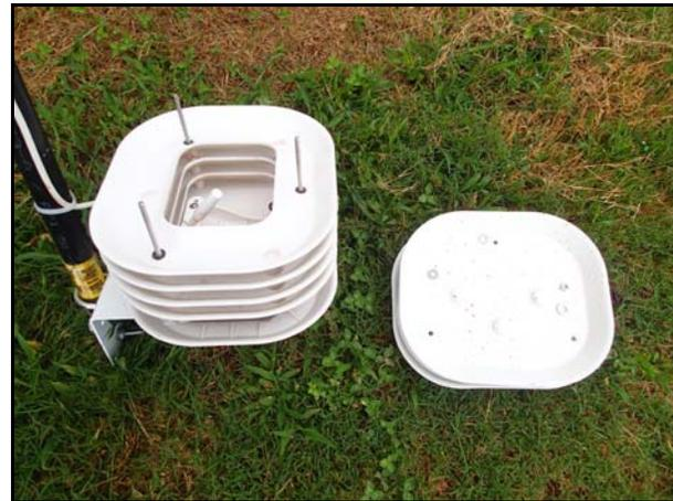
Figure 3. Partially assembled solar radiation shield with temperature sensor (upside down).
