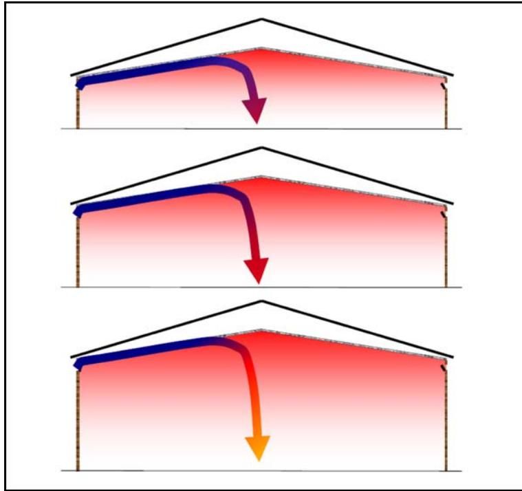
Figure 4. Warming of incoming air vs. Sidewall height.
