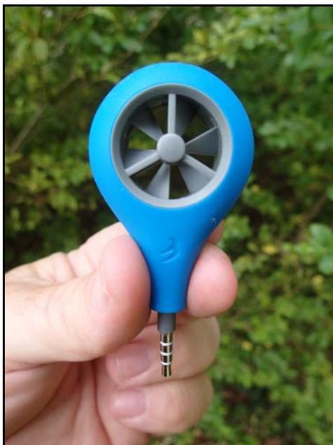
Figure 1. Weatherflow Wind Meter.
