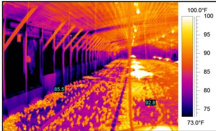
Figure 8. Leakage air leading to cool floors and reduced litter moisture removal
