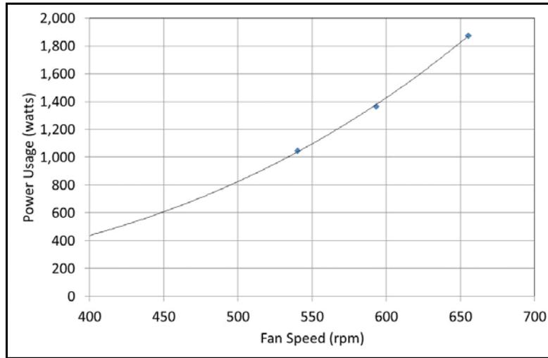
Figure 2. Fan power usage vs. fan speed.
