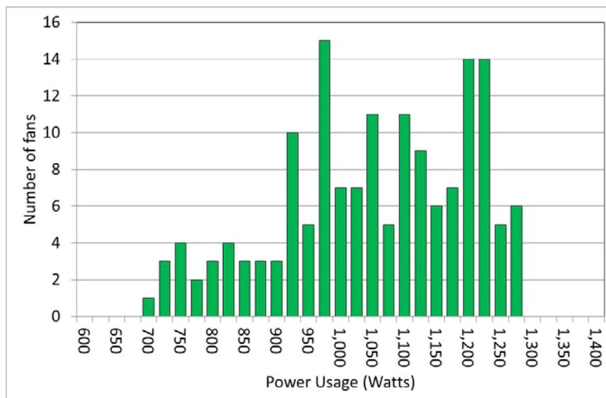
Figure 1. Power used by various 48" fans with 1 HP motors.
