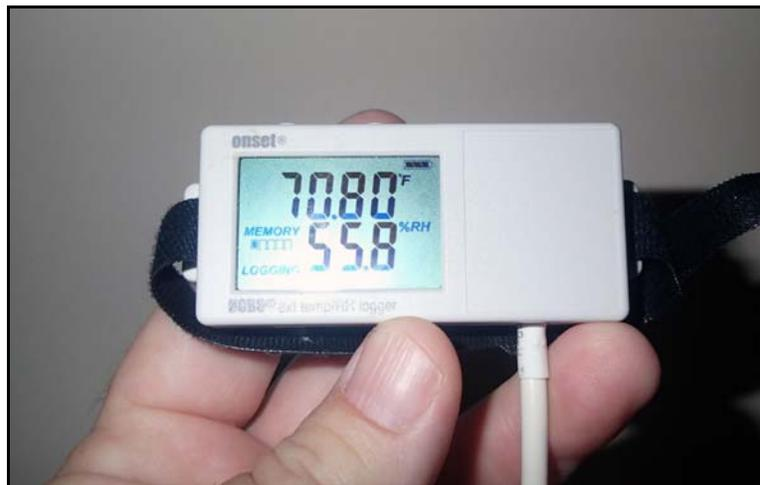
Figure 6. Onset UX100-023 temperature/Rh data logger
