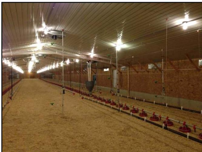
Figure 1. Anemometers poles used to determine a house's air velocity profile
