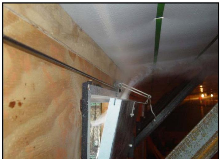
Figure 19. Smoke testing of galvanized door inlet open a small amount.
