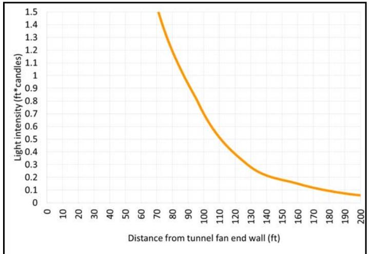
Figure 5. Light intensity vs. distance from tunnel fan end wall (tunnel fans in end wall).
