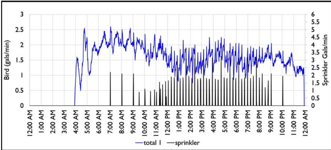
Figure 8. Bird and sprinkler system water usage (seven-week-old birds, 24 hours).
