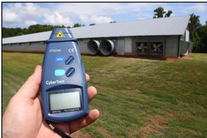
Figure 5. CyberTech DT2234A digital laser tachometer.
