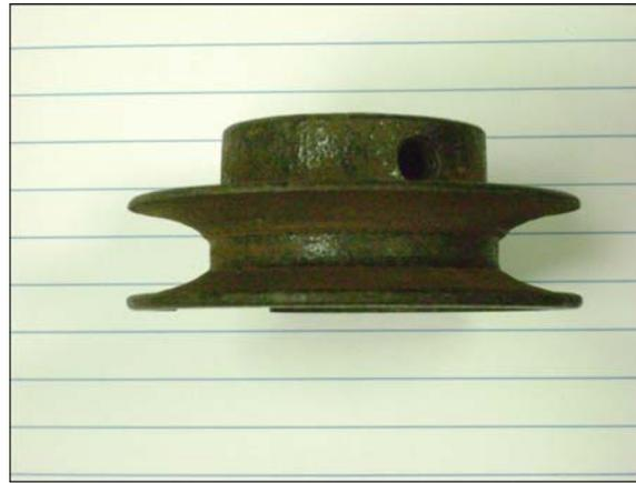
Figure 4. Worn motor pulley.
