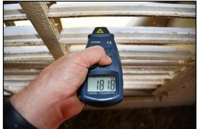
Figure 6. Using a laser tachometer to determine fan prop speed.
