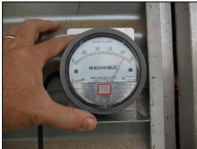
Figure 2. Magnehelic pressure gauge
