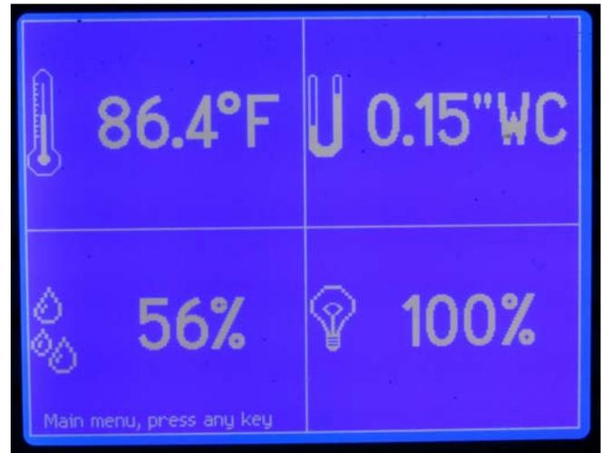
Figure 2. Poultry house controller displaying house conditions
