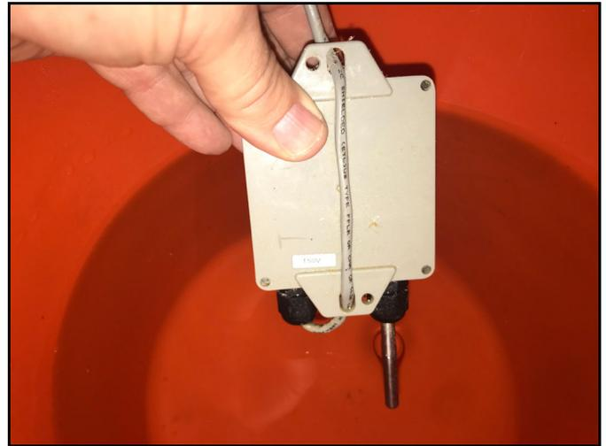
Figure 6. Placing controller sensor tip in water
