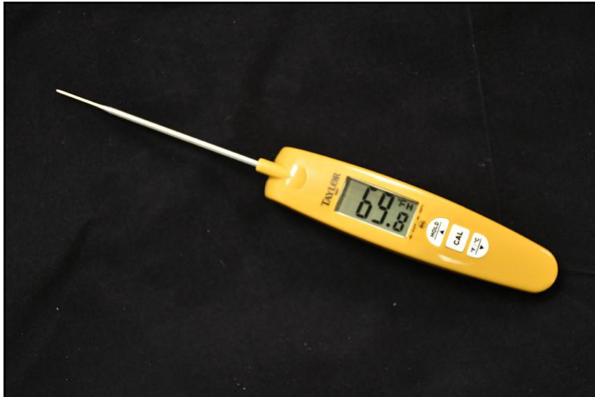
Figure 4. High accuracy food thermometer (Taylor 9867FDA Turbo Digital Pocket Thermocouple Thermometer)
