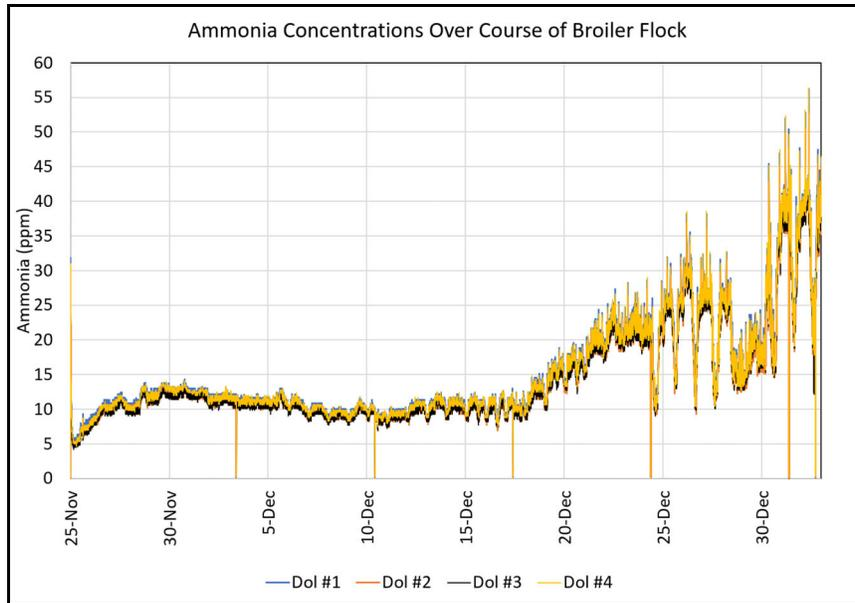
Figure 1. Broiler house ammonia concentrations as indicated by the four DOL 53 ammonia sensors
