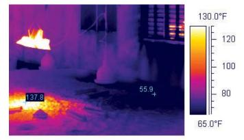
Figure 2. Draft from loose fan shutter
