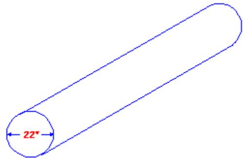
*Velocity =  $152,000 \text{ ft.}^3/\text{min.} / 380 \text{ ft.}^2$*
