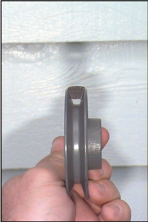
Figure 1. Belt riding at top of pulley
