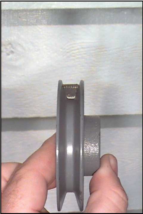
Figure 3. Worn belt riding in the bottom of the pulley.
