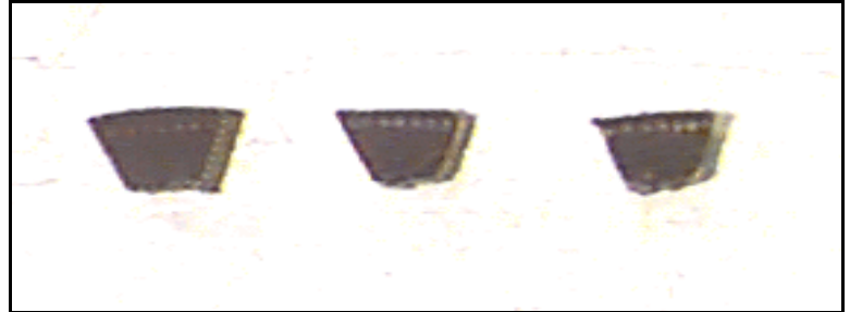
Figure 2. Fan belt becoming thinner over time
