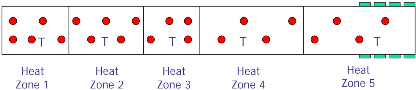
Figure 2. 500' broiler house with radiant brooders.
