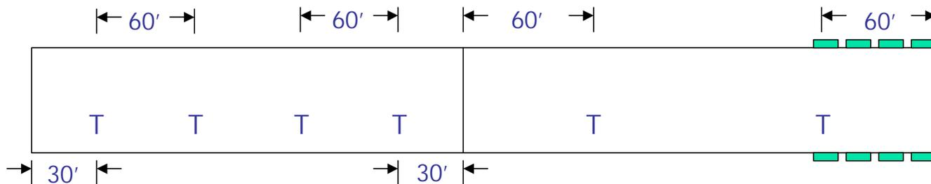
Figure 4. Temperature sensor placement in a 500' house with conventional brooders on the brooding end
