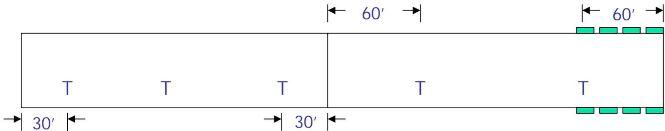
Figure 3. Temperature sensor location in a 500' house with radiant brooders
