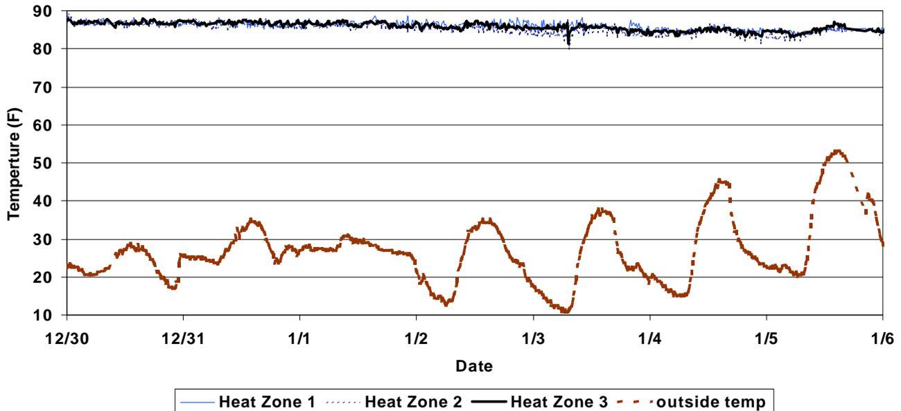
Figure 1. Tight temperature control during brooding
