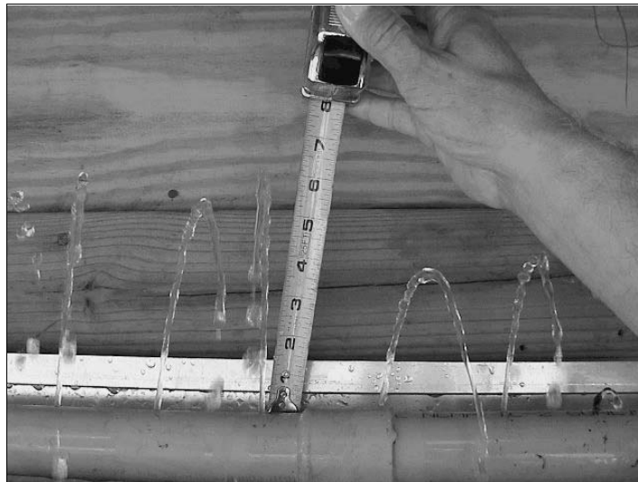
Figure 4. Measuring water column height
