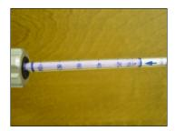
Though each tube is intended for a single measurement, multiple measurements can be obtained by subtracting the first measurement from the second measurement. It is important that the time between measurements be kept to a minimum because the chemicals within the tube quickly lose their potency after being exposed to air.
