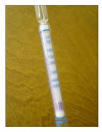
made to timer fan settings. Like the gas tubes, the accuracy of dosimeter tubes can vary significantly (+/- 10 to 20%) because of the difficulty involved with determining exactly where along the length of the tube the color changes from purple to beige, sampling procedure errors, as well as environmental factors.
