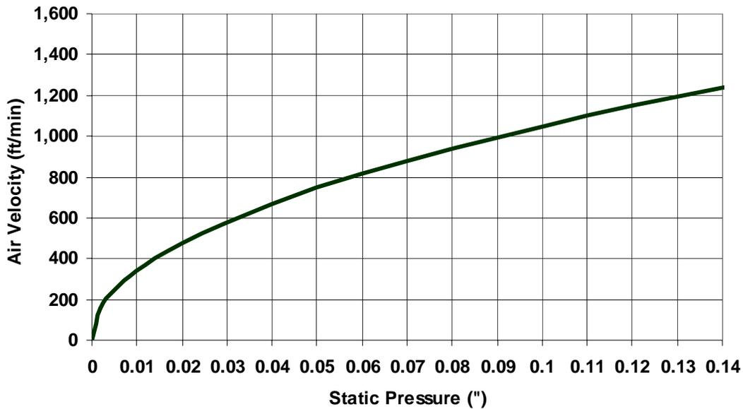
Chart 1. Approximate Air Speed Through an Inlet Opening Vs. Static Pressure.
