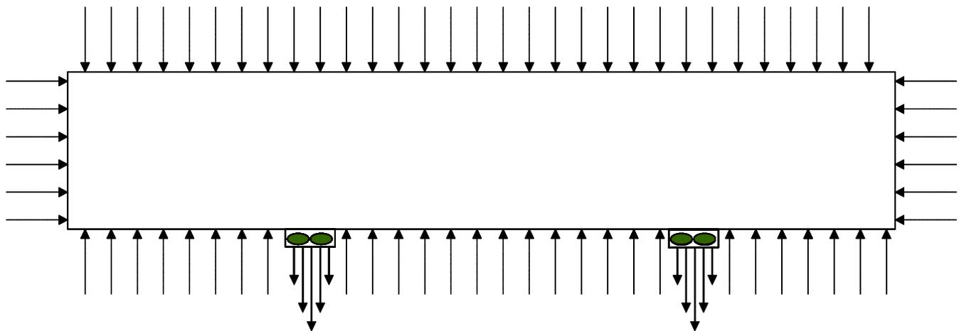
Figure 1. Consistent level of negative pressure throughout a house.
