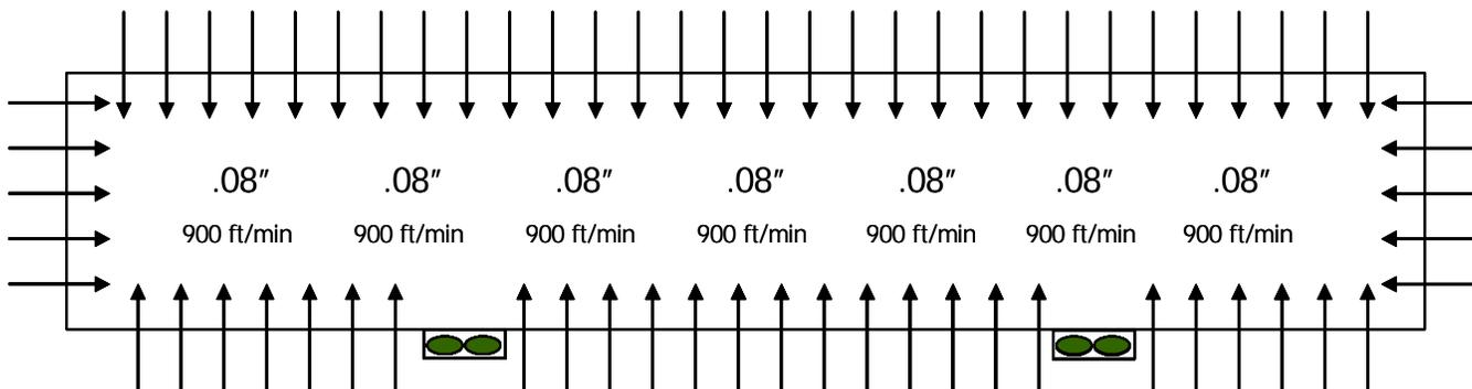
Figure 2. Even cracks in a house with a negative pressure.
