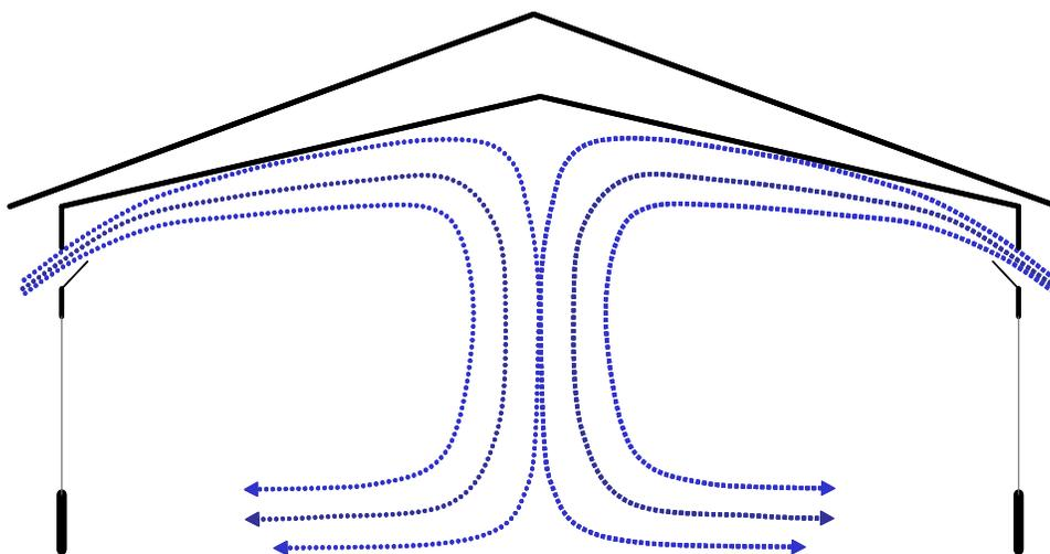
Figure 4. Inlet air flow in a house with a proper negative pressure.
