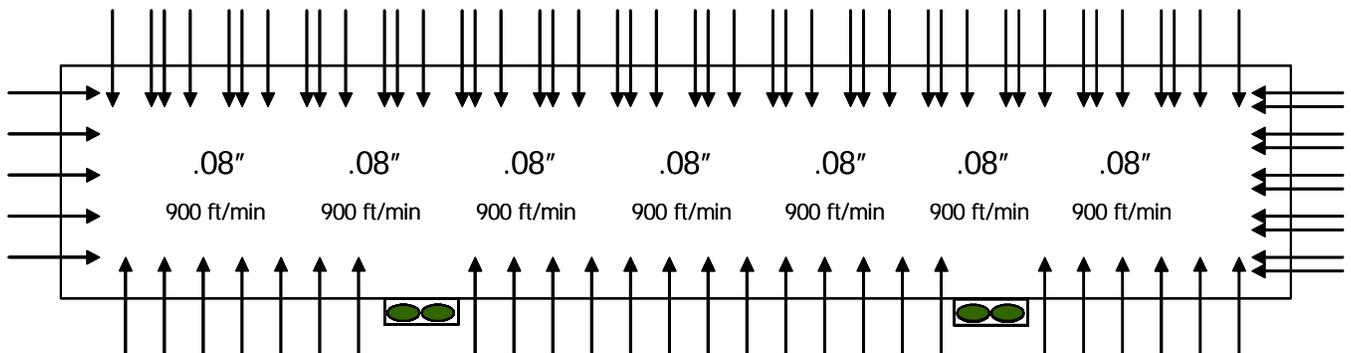
Figure 3. Uneven cracks/openings in a house with a negative pressure.
