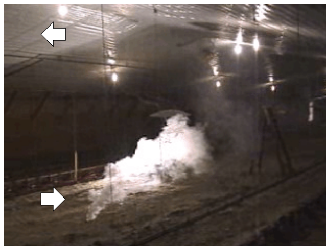
Figure 3. Air slowly flowing in opposite direction along the floor (arrows denote direction of air flow at the floor and the ceiling)
