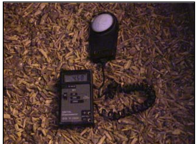
Figure 2. Light meter with sensor orientated toward light source.
