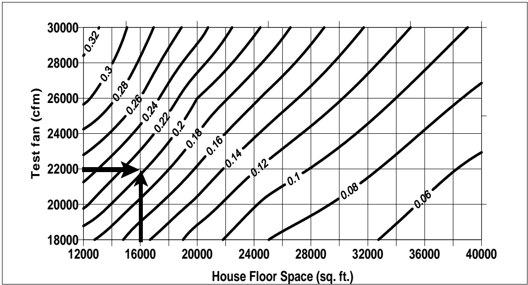
Figure 3. Minimum static pressure test reading based on fan cfm and house floor space.
