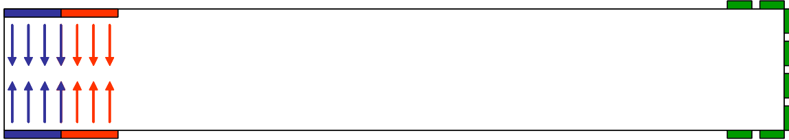
Figure 7. Split evaporative cooling pad system - Method 1.
