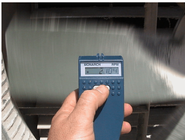
Figure 5. 54" Six-bladed tunnel fan (proper speed)
