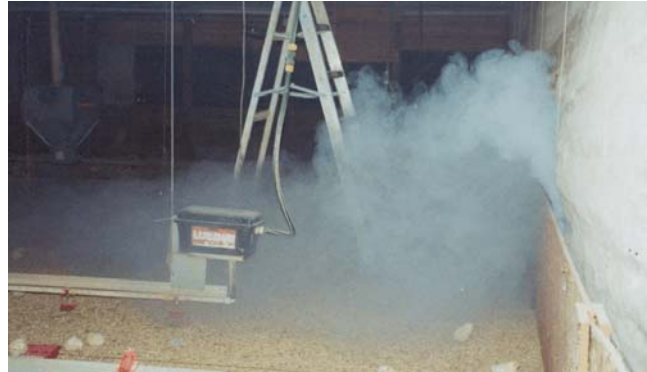
Leakage around brooding curtain from non brooding end of the house
