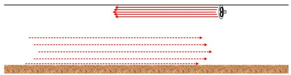
Figure 6. Counter-flow circulation pattern with fan blowing horizontal along ceiling.
