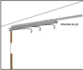
Figure 8. "Free" inlet air jet.
