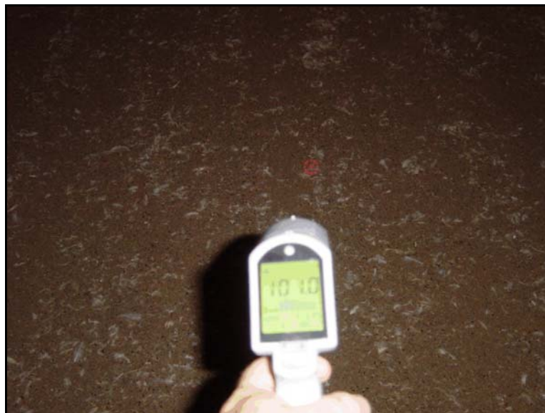
Figure 3. Non-contact thermometer with laser circle.
