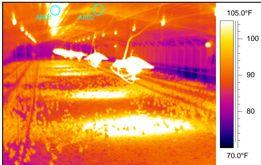
Figure 4. Reflected radiant heat from radiant brooders
