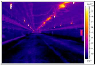
Figure 4. Thermal image of house using side wall inlets between flocks (summertime).
