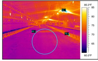
Figure 3. Thermal image of a house using attic inlets between flocks (springtime).
