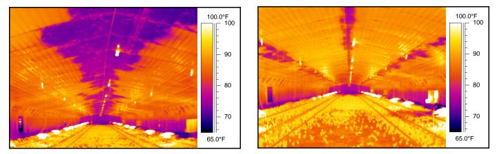
Figure 3. Thermal images taken during brooding in houses that were not reinsulated with the stabilized fiberglass insulation.
