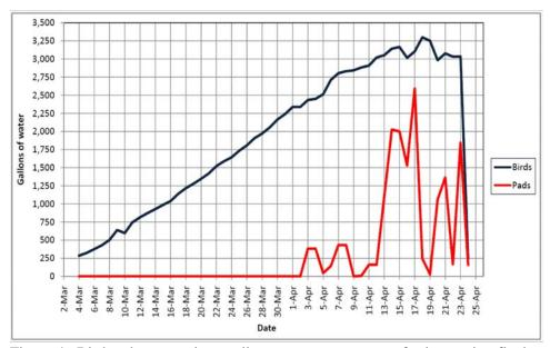
Figure 4. Bird and evaporative cooling system water usage for late spring flock.
