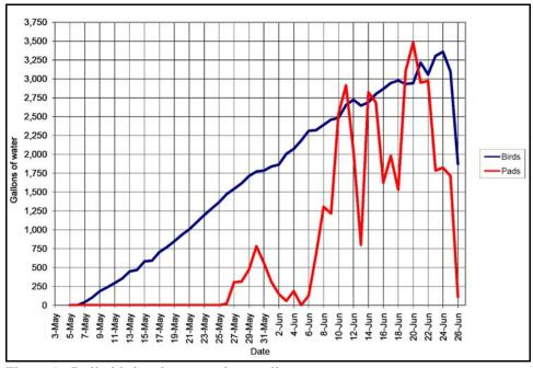
Figure 1. Daily bird and evaporative cooling system water usage.
