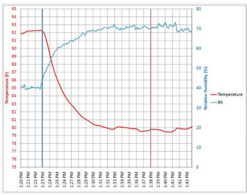
Figure 1. Cooling produced when air moves through a wetted pad.
