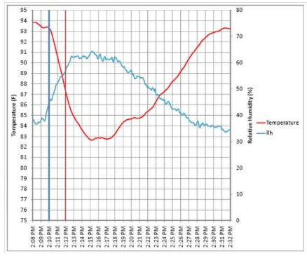
Figure 4. Water added to pads for two minutes.
