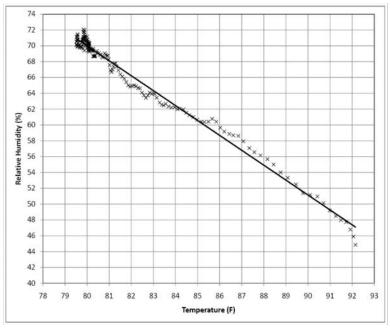
Figure 2. Temperature vs. Relative humidity of the air entering through a wetted pad.
