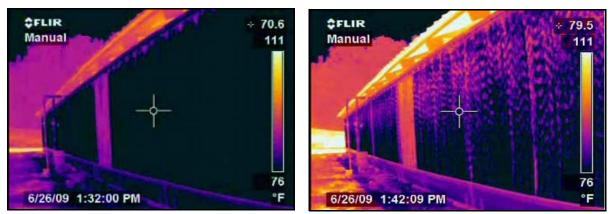
Figure 6. Thermal images of an evaporative cooling pad system.
