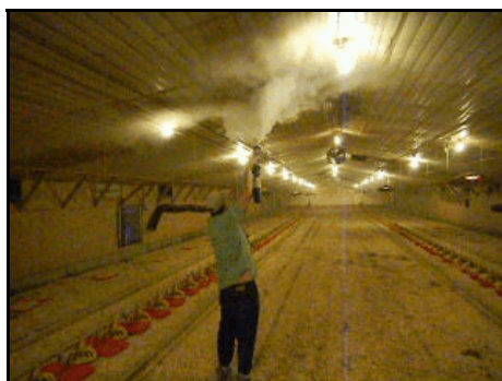
Figure 3. Smoke test of new four-way attic inlet.
