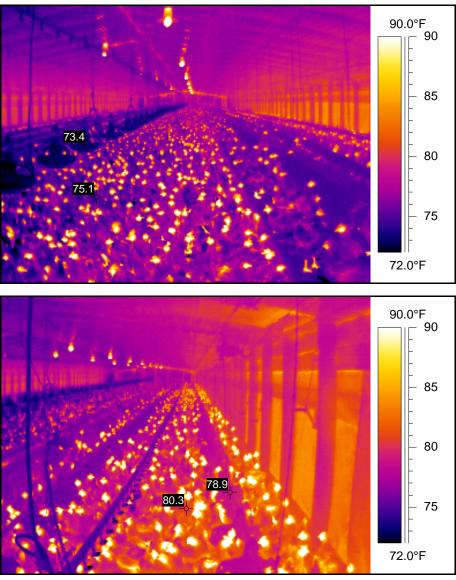
Figure 1. Thermal images of broiler-breeder house during mild weather (scratch area - top, slat area - bottom).
