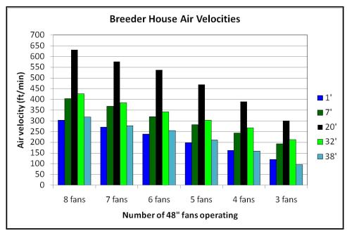
Figure 3. Air velocity profile in a 40' wide broiler-breeder house (18" above slats/ground).
