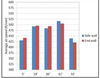
Figure 2. Average air velocity fans in the end wall vs. side walls.
