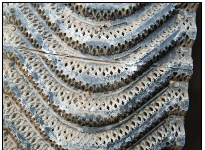
Figure 10. Interior of plastic pad after one year of use
